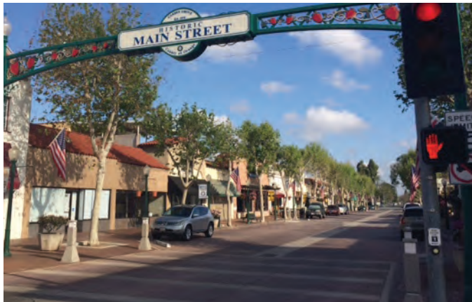
Example slow street - common elements include reduction or elimination of curbs and textured or colored surfaces
